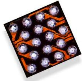
The IQS7222C ProxFusion® IC is a sensor fusion device for various multi-button applications. The sensor is fully I2C compatible and on-chip calculations enable the IC to respond effectively even in lowest power modes.
